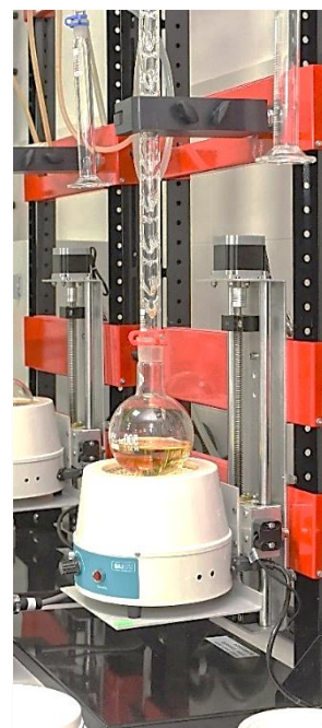
Details of vertical lift automatic actuator with platform for heating mantles
